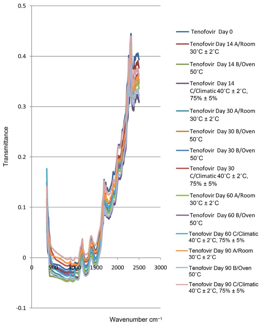
**Figure 1.** An overlay plot of Tenofovir disoproxil fumarate alone subjected at 40°C ± 2°C/75% ± 5%-Climatic chamber, 50°C-Oven and uncontrolled room conditions with 30°C ± 2°C, from Day 0 to Day 90.
