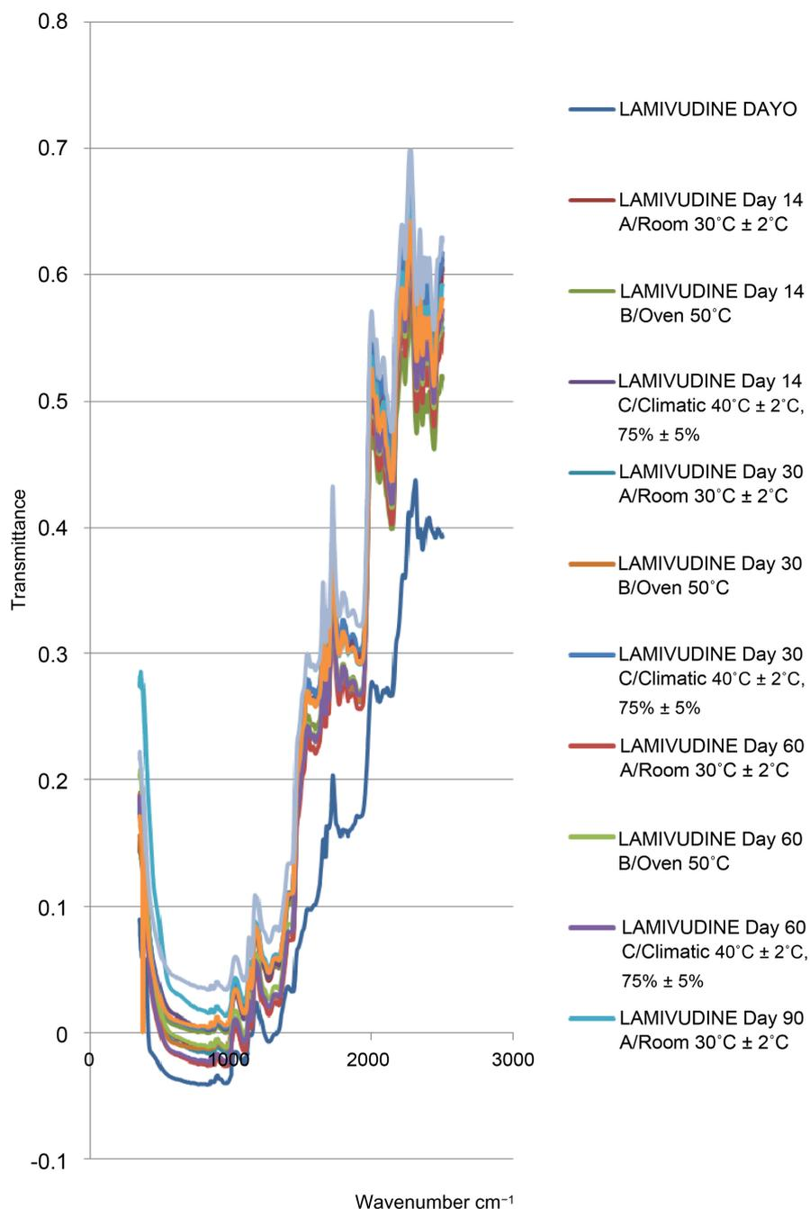
**Figure 2.** Overlay plot of Lamivudine alone subjected at 40°C ± 2°C/75% ± 5%-Climatic chamber, 50°C-Oven and Room uncontrolled room conditions with 30°C ± 2°C, from Day 0 to Day 90.
