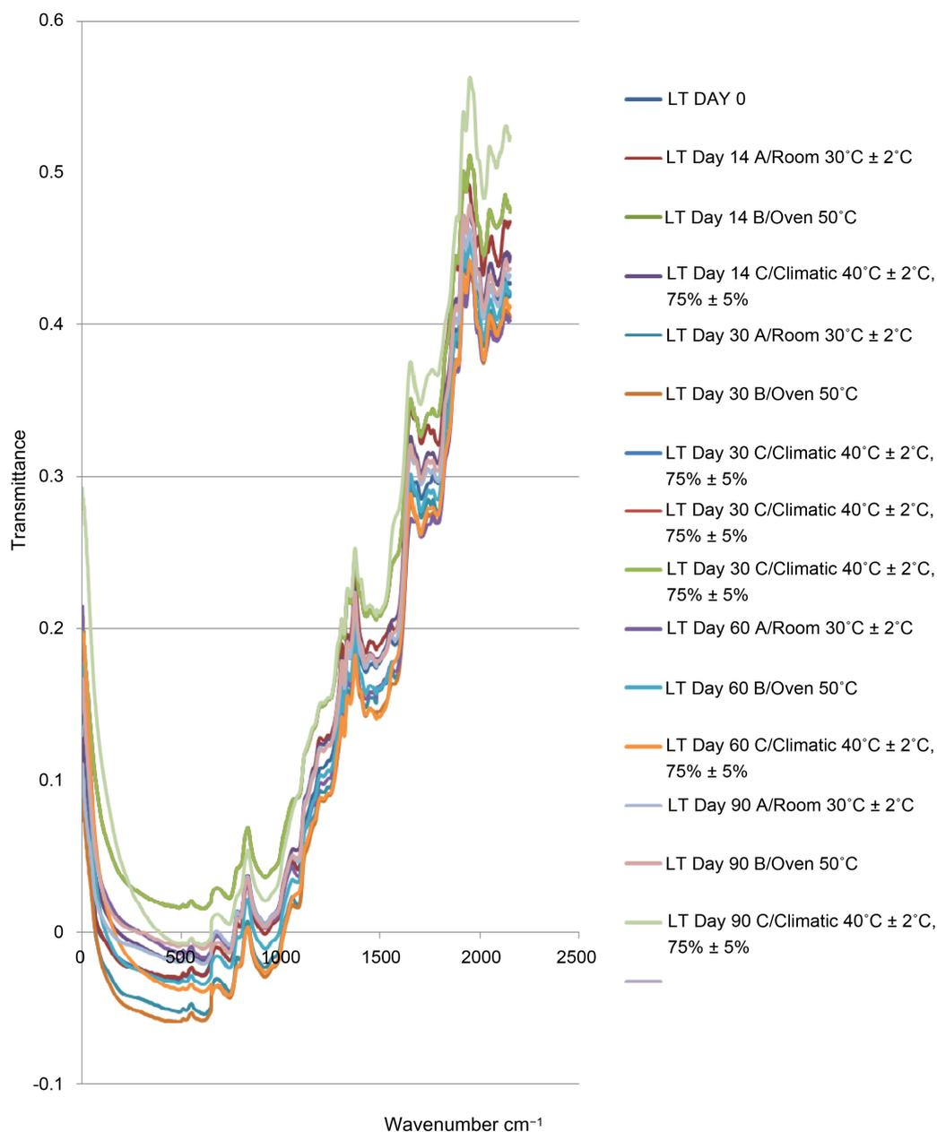
**Figure 3.** An overlay plot of Lamivudine and Tenofovir mixture subjected at  $40^{\circ}\text{C} \pm 2^{\circ}\text{C}/75\% \pm 5\%$ -Climatic chamber,  $50^{\circ}\text{C}$ -Oven and Room uncontrolled room conditions with  $30^{\circ}\text{C} \pm 2^{\circ}\text{C}$ , from Day 0 to Day 90.
