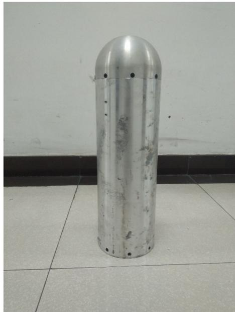
**Figure 1.** Designed flush air data sensing module.
