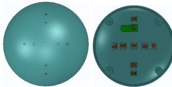
Figure 9. Installation position diagram of the pressure sensors.
