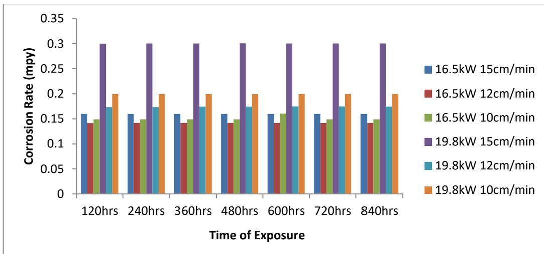
**Fig. 2. Corrosion rate of plain face welded samples at different power input and welding speed in tetraoxosulphate (VI) acid solution**
