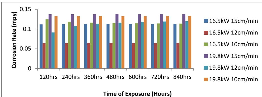
**Fig. 3. Corrosion rate of double-v edge welded samples at different power input and welding speed in tetraoxosulphate (VI) acid solution**
