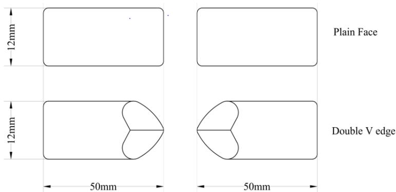
**Fig. 1. Shapes of the low carbon steel welding samples**
