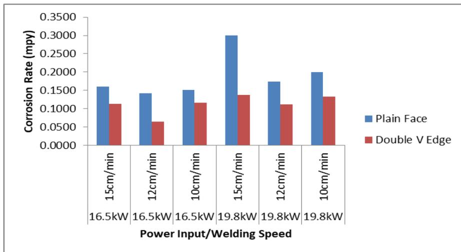
**Fig. 4. Average corrosion rates of both plain face and double-v edge shape welded samples at different power inputs and welding speeds in  $H_2SO_4$  solution**
